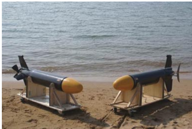
Figure 7. The comparison UUV (with propeller, left) and SPC-III biorobotic UUV (with fin, right) settled in cradles on the beach.
