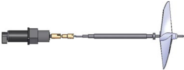
Figure 3. Mechanical configuration of the screw propeller.
