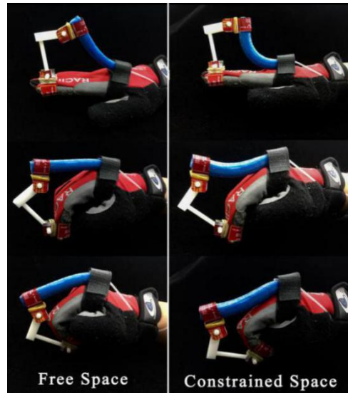
Fig. 6 Snapshots of the index finger and the glove. a) Simulating the free space. b) Simulating the constrained space.
