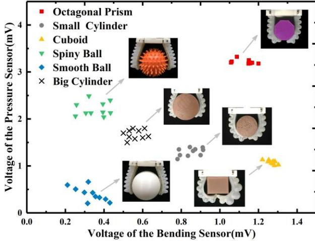
Figure 6. Clustered sensory data for enveloping grasps. Ten grasps were conducted for each object. The gripper was fully softened during the experiment. See supplementary video for more details.
