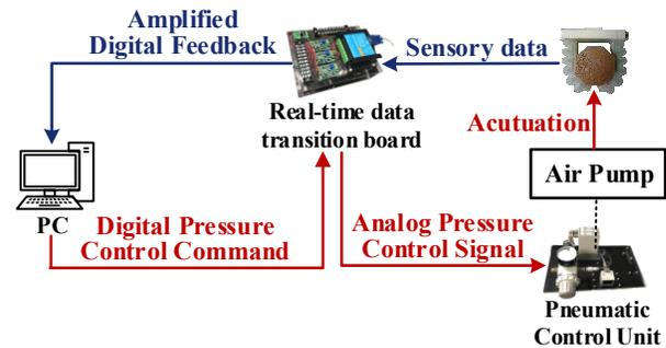
Figure 2. Pneumatic control system for the soft actuator on which most of the experiments were carried out. The pneumatic control unit is composed of proportional air valves (ITV0030, SMC, Japan), air pressure sensors (ISE30A-01-C, SMC, Japan) and a pressure gauge.
