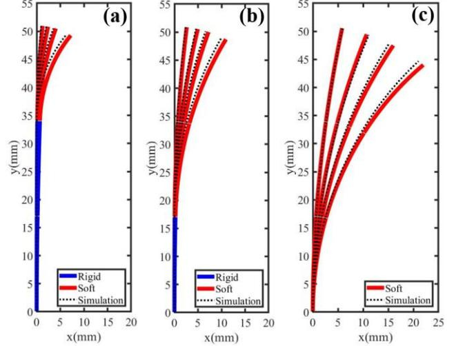
Figure 7. Comparisons between experimental results and model-based simulations of closed-loop control of the soft gripper under different DoF configurations.
