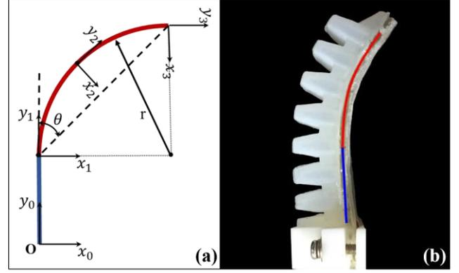
Figure 4. Kinematics model of the gripper. (a) PCC kinematics model of the gripper. (b) Corresponding DoF configuration of the prototype.
