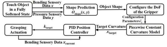
Figure 3. Flow diagram of model-based object grasping under the condition of unknown shape of the object.
