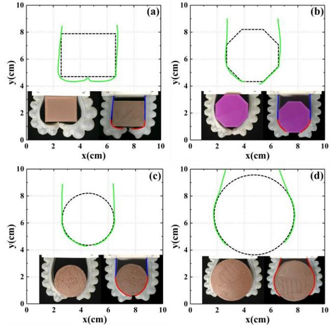
Figure 8. Grasping Verifications of objects with different shapes. In each subgraph, the picture at bottom left shows the enveloping result of the gripper in a fully softened state, while the picture at bottom right represents the improved enveloping performance of the gripper under a specific DoF configuration.
