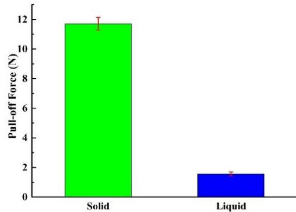
Figure 8. The pull-off force comparison of the two grippers. “Solid” means the average value when the LMPA was in the solid state while the gripper grasped the object, while “Liquid” means the average value when the LMPA was in the liquid state for gripping.
