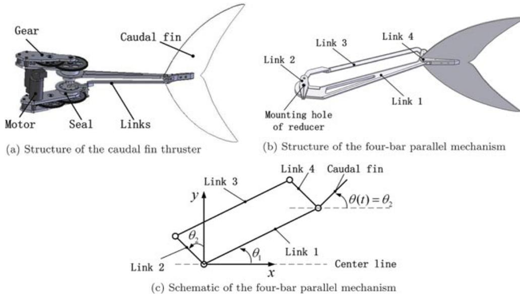
Figure 4. Mechanical configuration of the caudal fin thruster.
