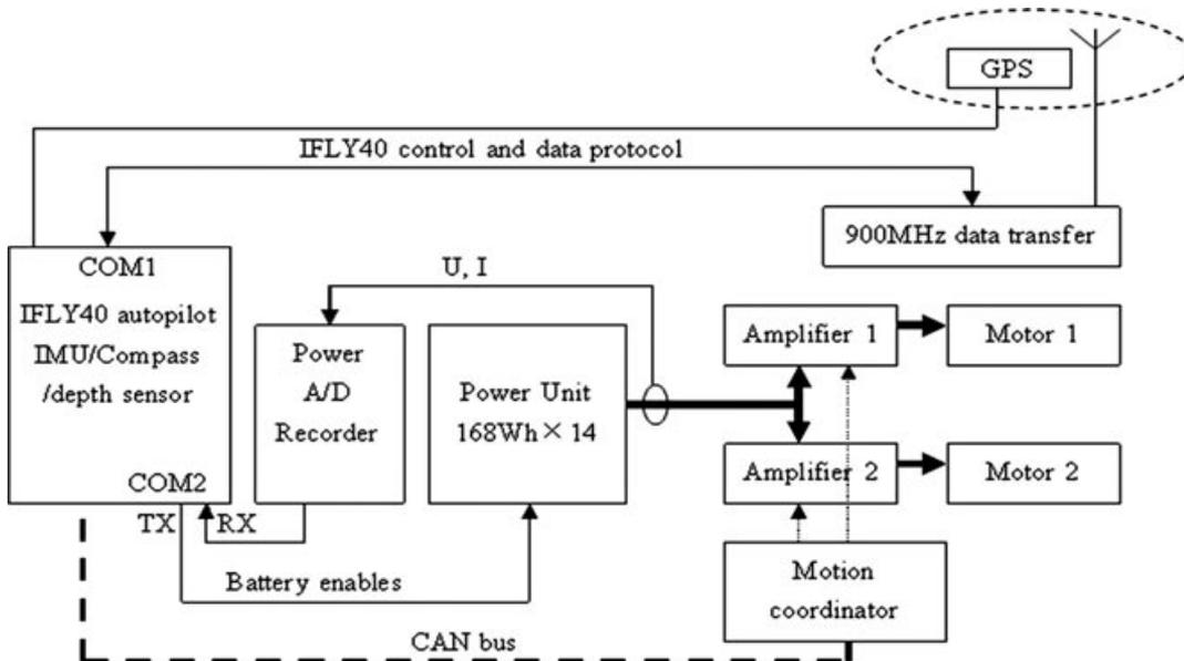
Figure 6. Electrical system of SPC-III robotic fish.
