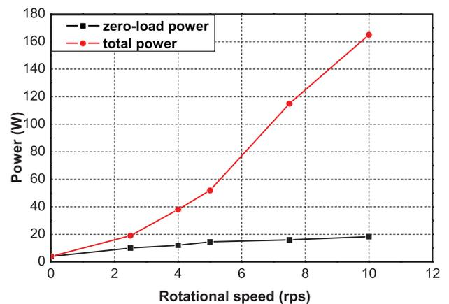
**Figure 9.** Zero-load and total power of screw propeller.
