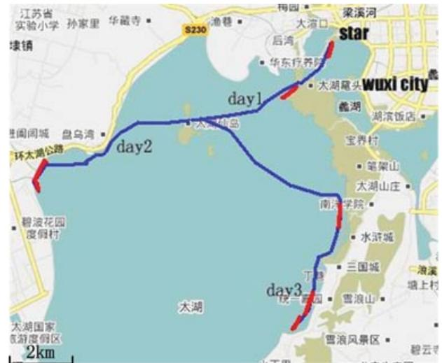
**Figure 13.** Cruising trajectories of SPC-III in the water quality probe experiment at Taihu Lake are shown in blue, and the areas under heavy pollution are indicated in red.
