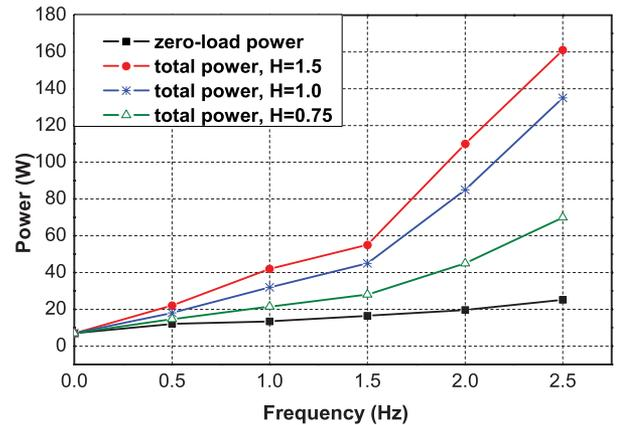
**Figure 8.** Zero-load and total power of caudal fin.
