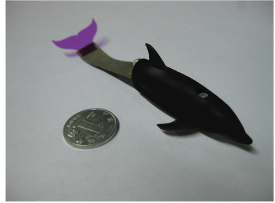
Figure 1. Prototype of the robotic swimmer.
